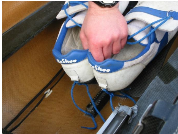
Fig 3: Checking that the heel restraints are connected.
