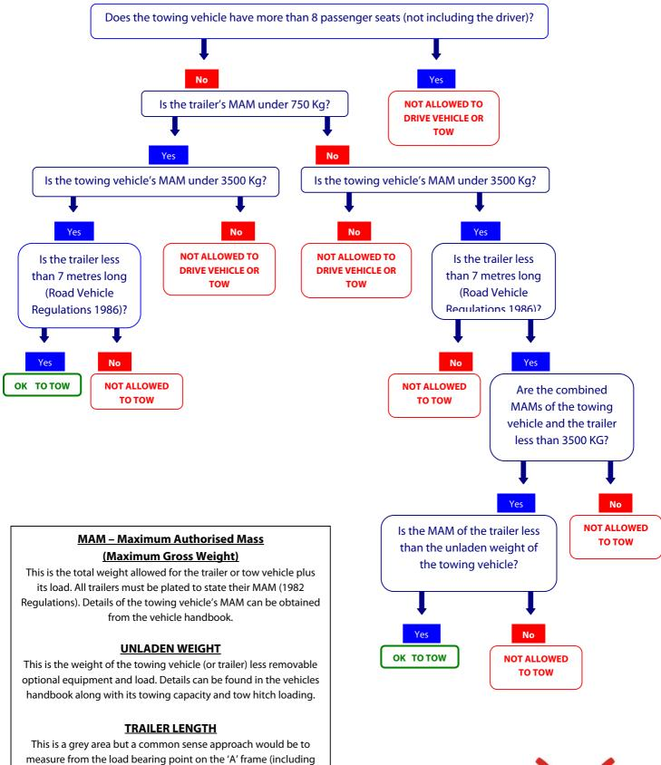
attached boxes etc) to the rear lighting unit on the extended draw
